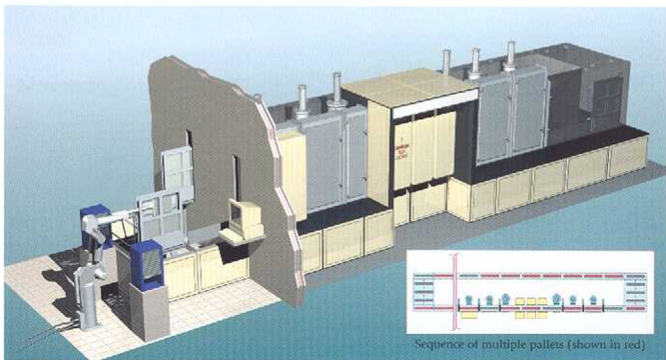
HANDS OFF—A robot arm loads a pallet onto the pallet carrier as it prepares to unload a processed pallet at the return exit. This three-dimensional rendering depicts one possible configuration with load and unload stations, load-locks, pumping chambers, process chamber, and return carrier.
