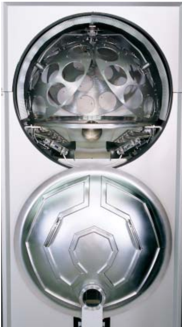
UP AND DOWN—Slide-down door minimizes valuable clean room floor space requirements.
